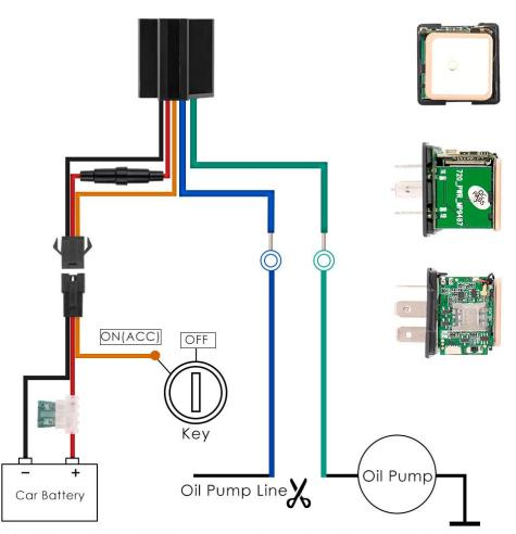
NOTE: Working voltage: 10-40V DC , please find professional repair man or 4S store to install the device!
