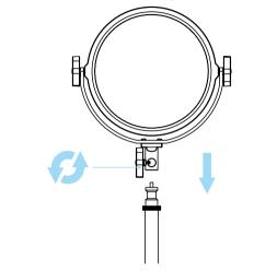
3 Loosen the adjustment knobs on both sides of the U-bracket, adjust the angle of the panel you need, and then tighten the adjustment
