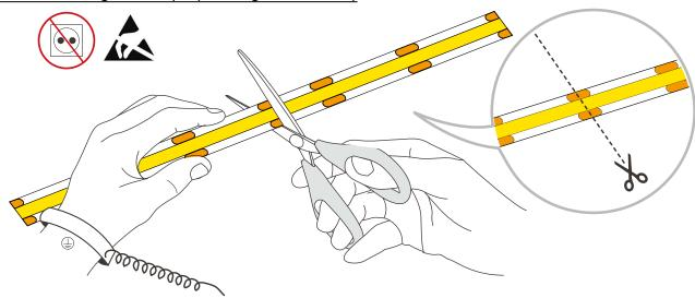
Calculate the needed length and cut off the extra length along cutting mark if necessary; If need to add wires, please weld them at the next location with printed mark.
