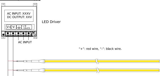
Notes: please make sure the "+" and "-" of the product input correctly connected to those of the power supply output.
