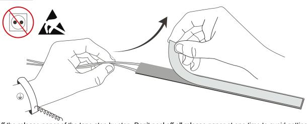
peel off the release paper of the tape step by step. Don't peel off all release paper at one time to avoid getting your strip in a mess.
