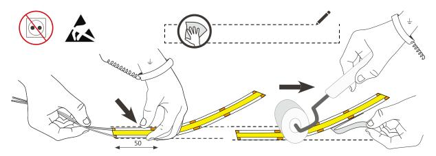
Stick Mylar tape to isolate the cutting position from the object surface, then press the strip which sticking on the surface.
