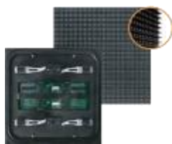
SMD LED Lights
