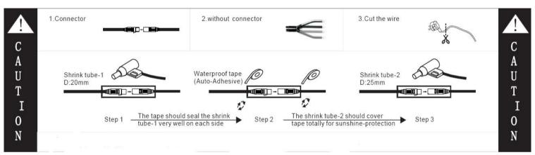
Neglect on action of the above treatment will lead to failure of waterproof and proper work of the lights. Water can be sucked into the fixture via interior pipe of the cables after light be switched off, due to minus pressure!!!
