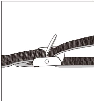
Position the Wildlife Camera as desired and pull the loose end of the securing strap tight until the camera is firmly secured.
