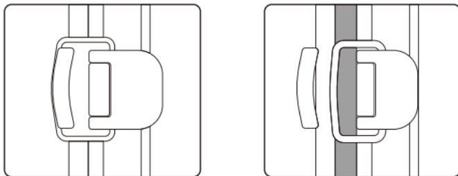
A fixing for a padlock is provided between the two locking brackets, allowing the camera to be securely locked.
