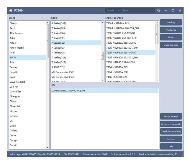
After selecting the correct ECU model, the "Platform" button will appear on the right. As shown in the figure above, click the "Platform" button to enter the ECU
