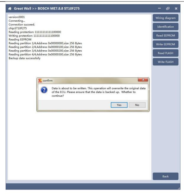
Note: in the process of writing data, it is strictly forbidden to disconnect the power supply or the connection of the device; if the software is shut down or the computer is shut down or crashes unexpectedly in the process of writing data, please do not disconnect the power supply or the connection of the device, and keep it for 15 minutes. The device can recover the data independently.
