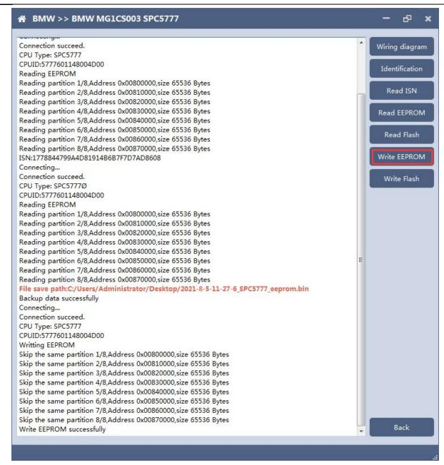
Note: During the data recovery process, it is strictly forbidden to disconnect the power supply or disconnect the device, otherwise it may cause ECU damage; if the software is shut down unexpectedly or the computer is shut down or crashed unexpectedly during the data recovery process, please do not disconnect the power supply or device Connect for 15 minutes, and the device can complete data recovery independently.
