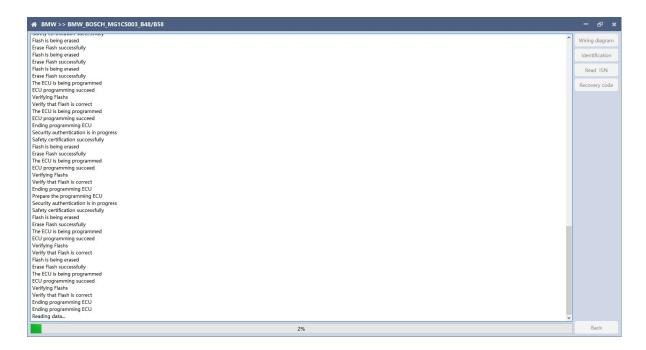
After the programming is completed, if there is a coding file before the ECU programming, the coding recovery will be performed automatically. After programming, the software starts to read data, as shown in the figure above.
