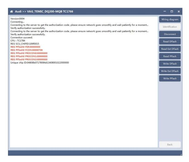
After connecting to DQ200, the "identify" button will be grayed out. You can proceed to the next step. When you click "disconnect", you can identify again.
