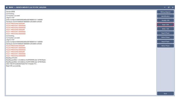
Click the "Read ISN" button to start reading the ISN. Wait for a while to complete the reading of the ISN.
