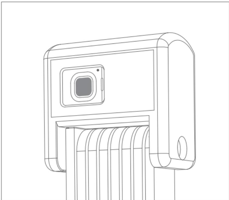
Long press the fingerprint board for about 5 seconds to turn on/off the Bluetooth of ZiiLock. When the lock beeps with a red light, the Bluetooth of the lock is turned off.
