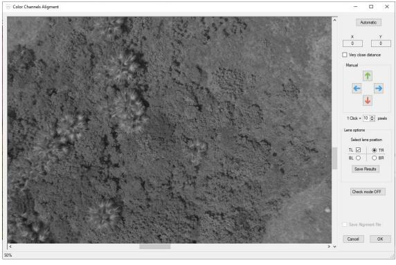
Check the alignment by identifying a distinctive point in the image and use the arrows to move the quadrants' images for optimal overlapping.
