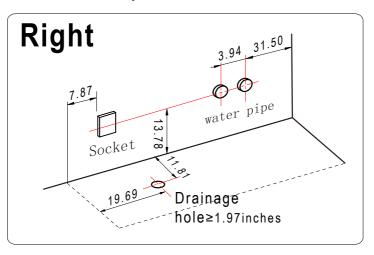
A Notice The safe distance between power supply and water supply should be not less than 30cm.
