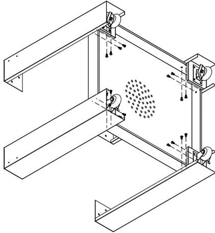
2/. Fasten legs on the oven body with 12pcs of 1/4"\*15mm screws
