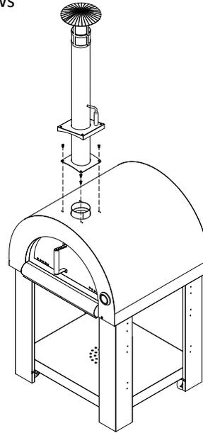
6/. Installed chimney cap with 4pcs of 5/32"\*10mm screws
