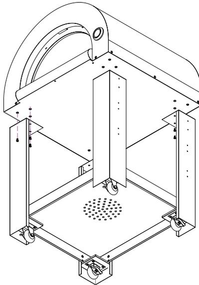
3/. Ash support installment with 4pcs of 1/4"\*15mm screws
