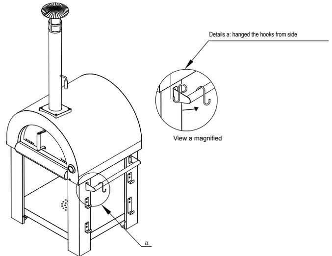
10/. Installed 3pcs of hooks 1 and 1pc of hooks with 8pcs of 1/4" \* 15mm screws
