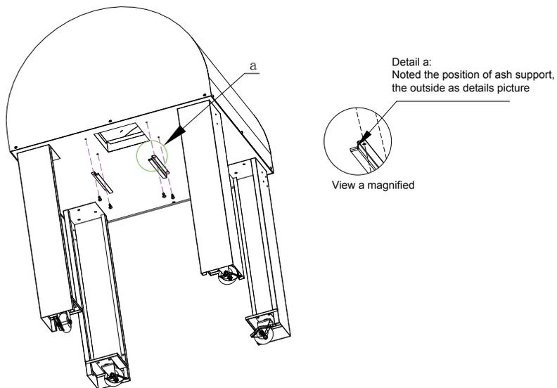
4/. Installed the ash box on the oven bottom
