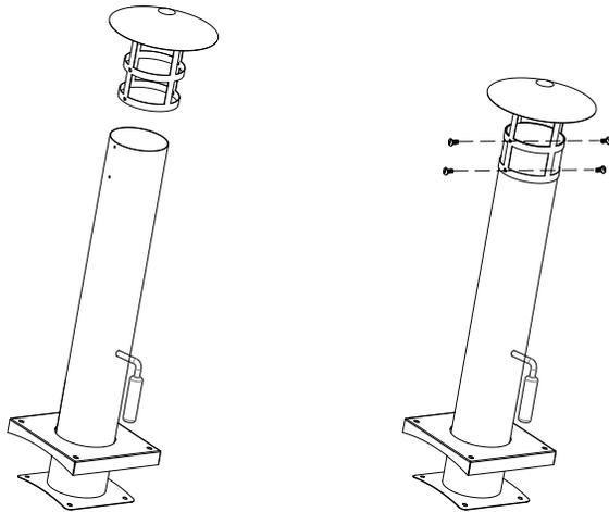
8/. Installed chimney box with 4pcs of 1/4" 30mm screws
