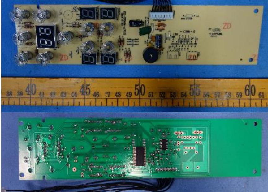
Control PCB view of model GK-CF246004(similar to models GK-CF246404,GK-CF306704 )
