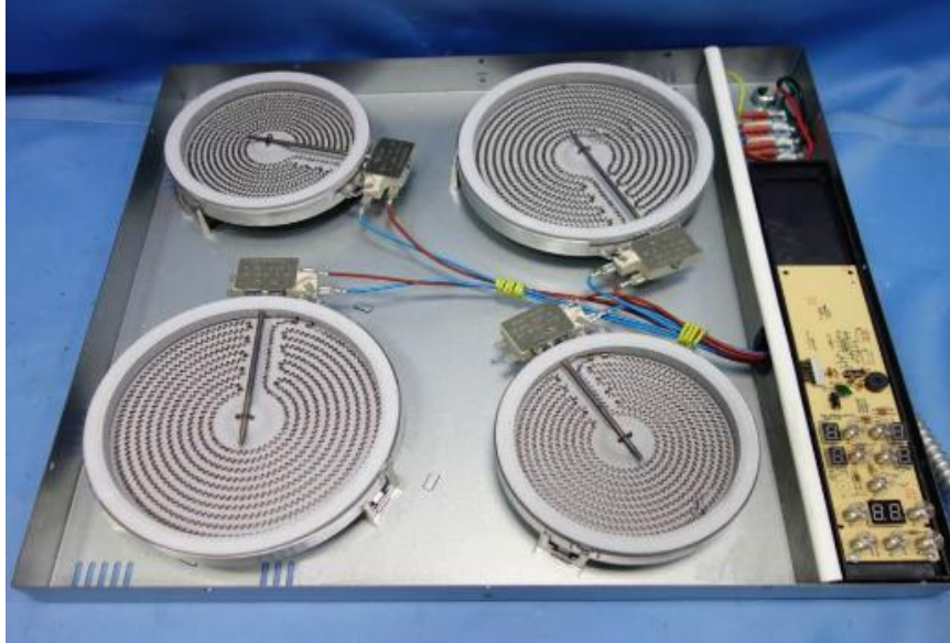
Internal view of model GK-CF246004 (similar to model GK-CF246404,GK-CF306704 )
