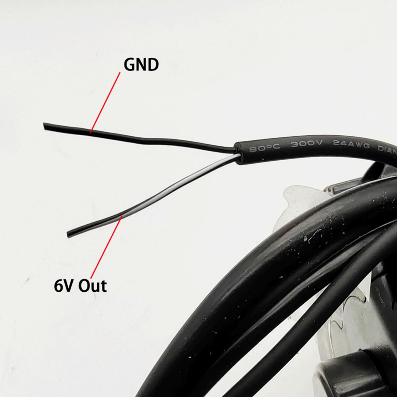
We can modify the original plug, For better contact and simple waterproofing You can also omit this step
