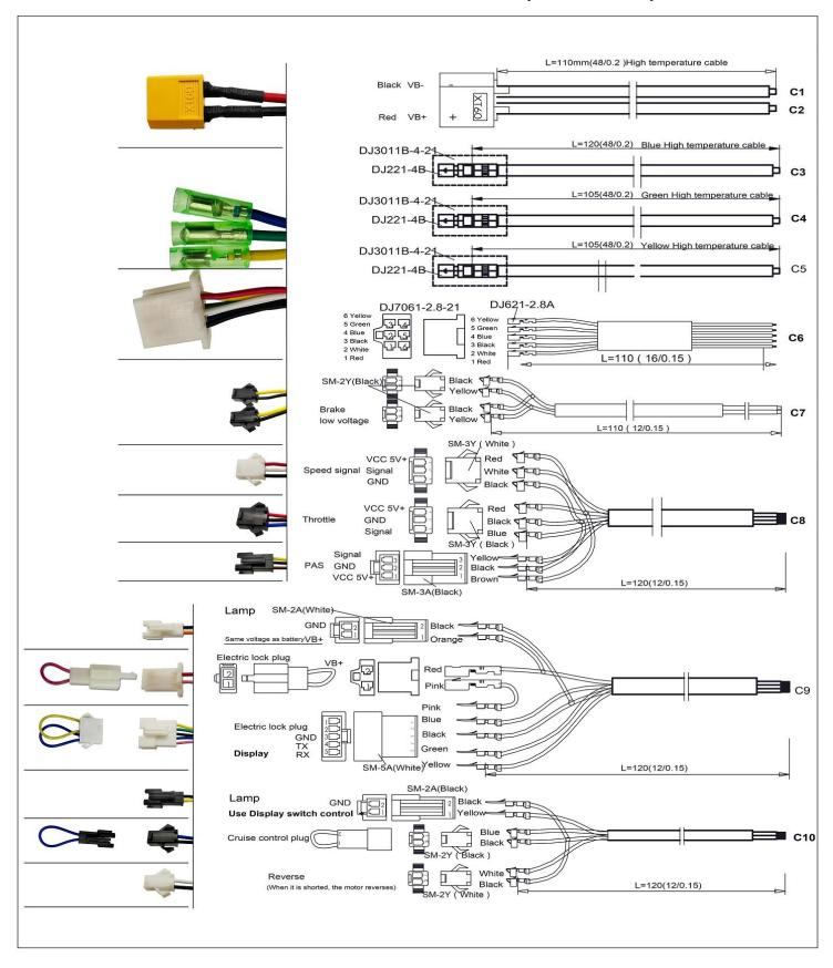
1. Power Supply/Power Input Connection, XT60 Male Plug: C1, C2
