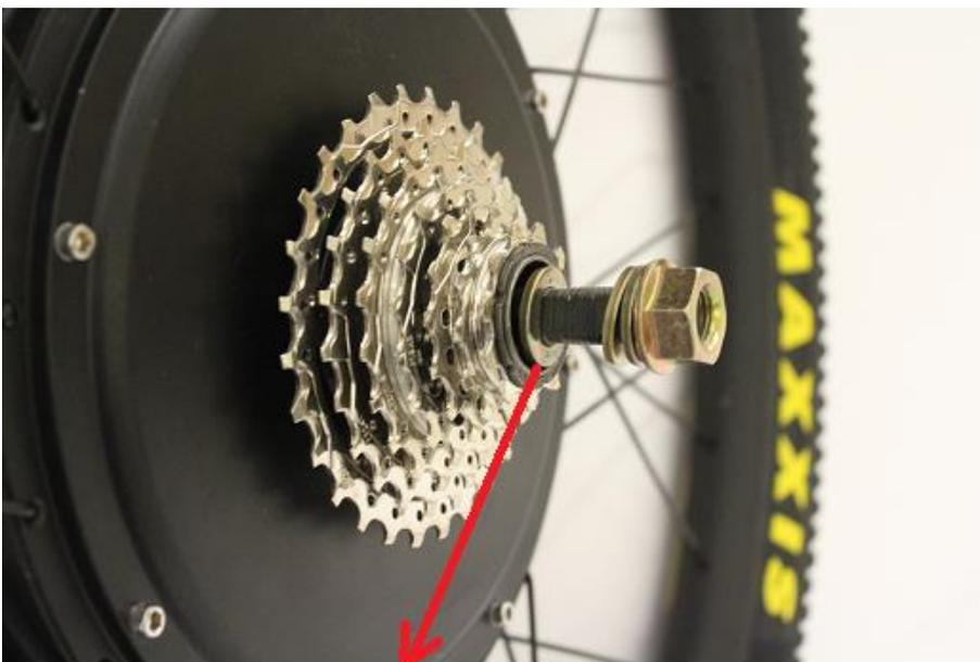
**Please also put a washer at freewheel side, between freewheel and fork, so that fork will not press cassette bearing**
