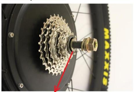
Please also put a washer at freewheel side, between freewheel and fork, so that fork will not press cassette bearing
