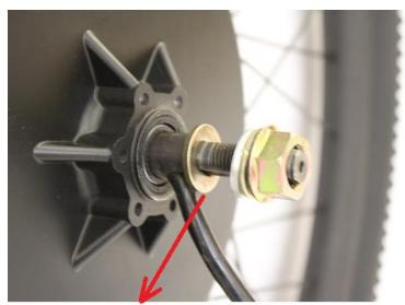
If the distance between rotor and rear fork is less than 15mm, then please put a washer between motor axle and fork to adjust the distance.
