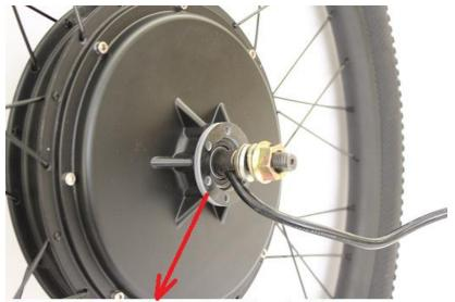
If your hydraulic disc brake caliper is thick, you may need to put a washer here to add distance between brake rotor and motor
