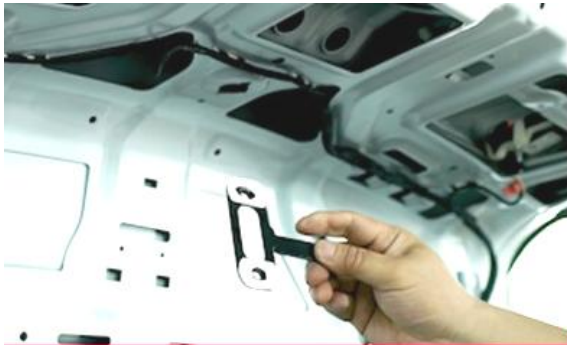
11.ADD THE STIFFENER IN TRUNK BACK SIDE
