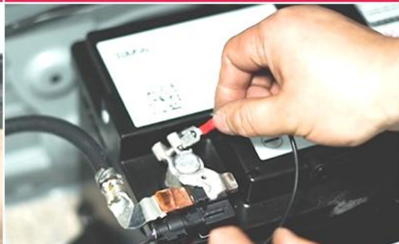
15. FINAL CONNECT POWER BATTERY
