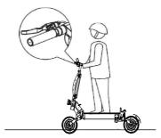
6 Press the brake lever to brake, and gently press the rear fender to assist the brake.
