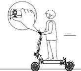
4 Press the THROTTLE button slightly on your right hand to start and rotate the handle to turn
