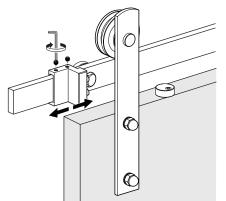
Install the floor guide. Put floor guide on the floor first to fix a suitable position and make a mark so that the tip of the floor guide can work well in the slot.
