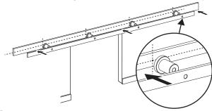
Insert door stoppers into rail. Install door stoppers between A-B and C-D. Door stopper is used to prevent the hangers coming out of the rail.
