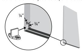
Install the hangers onto the door according to the measurement in the pictures below.
