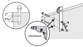
The rubber ends are used to protect the door from touching the rail when sliding the door. You need to drill holes on the door top side, please drill the holes ½" away from the edge of the door. Then install the rubber ends on the door.
