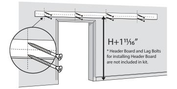
Place the rail against the wall, and use a pencil to mark where the holes should be.
