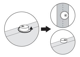
Adjust the 2 door stoppers to find a suitable position, Use the hex key to screw the door stoppers in place.
