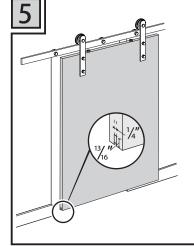
5. Use router or circular saw to create a kerf at bottom of the door, along the center to allow the tip of the T-shaped floor guide to fit in between, to keep your door stable and prevent the door bottom swinging back and forth when you slide it open and closed.
