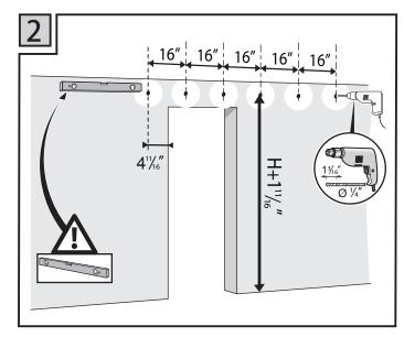
2. If you install the rail onto concrete wall, use Drill bit to drill hols on the wall where pencil mark is. If you install the rail onto wood stud, there is no need to drill holes in this step.
