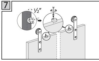
7. The rubber ends are used to protect the door from touching the rail when sliding the door. You need to drill hols on the door top side, please drill the holes  $\frac{1}{2}$  away from the edge of the door. Then install the rubber ends on the door.
