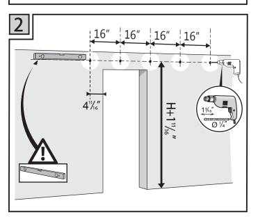
2. If you install the rail onto concrete wall, use Drill bit to drill hols on the wall where pencil mark is. If you install the rail onto wood stud, there is no need to drill holes in this step.
