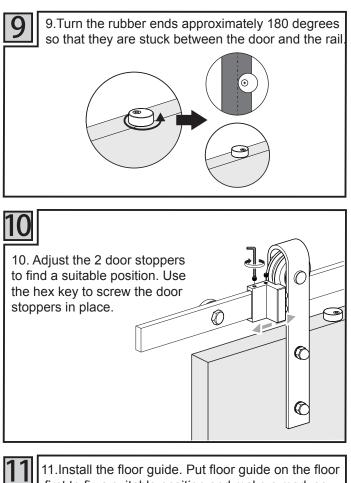
11.Install the floor guide. Put floor guide on the floor first to fix a suitable position and make a mark so that the tip of the floor guide can work wee in the slot. Use drill bit to drill holes on the floor where the mark is, and then install the floor guide.
