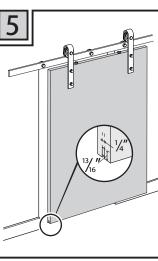
5. Use router or circular saw to create a kerf at bottom of the door, along the center to allow the tip of the T-shaped floor guide to fit in between, to keep your door stable and prevent the door bottom swinging back and forth when you slide it open and closed.
