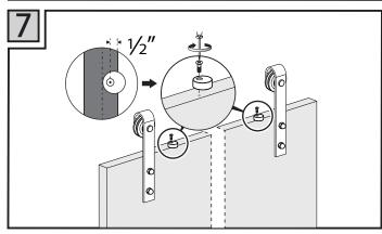
7. The rubber ends are used to protect the door from touching the rail when sliding the door. You need to drill hols on the door top side, please drill the holes 1/2" away from the edge of the door. Then install the rubber ends on the door.
