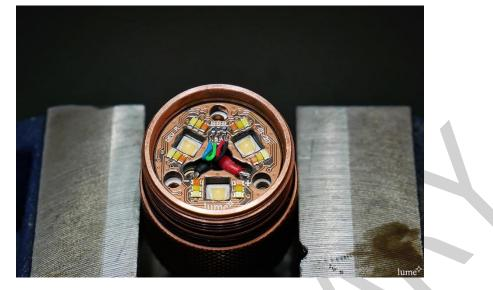
Finally, the four wires are soldered onto the pads. The above photo shows an example of an assembled tri-LED AUX board in a FW3C. The wire connected to COM should be soldered into the pad labeled K on the AUX LED board; this pin is the common cathode of the 3 LED banks. RED, GREEN and BLUE is connected to R, G, and B respectively.
