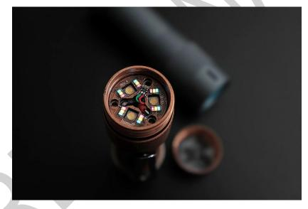
After installation, the AUX LEDs should illuminate by default when a battery is inserted. If the AUX LEDs do not come on, check that they are not disabled in the firmware – if they are, they can be easily re-enabled. See section 7.1 for instructions. Otherwise, ensure that the LEDs are installed correctly, and that the wires are soldered correctly.
