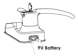
Your Lockly<sup>™</sup> will automatically detect battery polarity. So hold your 9V battery lead in place against bottom of the Lockly<sup>™</sup> to **temporarily** activate the screen to enter your **Access Code**. Be sure to hold the 9V battery against the contact points located at the bottom of the lock until you have successfully unlocked your door with your **Access Code**. Once unlocked, batteries should be replaced immediately.
