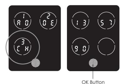
While in **Programming Mode**, select "**3CH**" to check registered **Access Codes.** If you are not in **Programming Mode**, please see Section 3.2 to enter **Programming Mode**.
