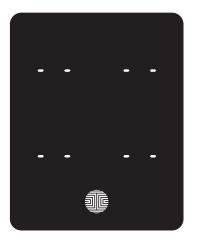
If there are no **Access Codes** registered in your smart lock, **Check Access Code** mode will be invalid. The default **Access Code** will not be shown on the display keypad, and you will see the following screen shown to the left instead.
