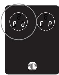
While in **Programming Mode**, select "**2DE**" to delete an **Access Code**. If you are not in **Programming Mode**, please see **Section 3.2** to enter **Programming Mode**.
