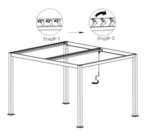
Turn the position from step9-1 to step9-2 first, then assemble the shutter.
