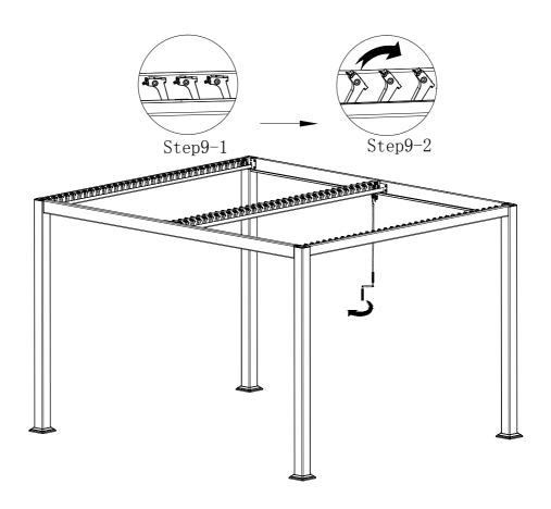
Turn the position from picture 1 to picture 2 first, then assemble the shutter.
