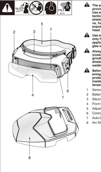
The auto-darkening goggles provide eye protection only. Use additional personal protection equipment shield, face shield, balaclava, hard hat, etc.) to shield exposed skin and protect
