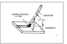
Fig 22 Angles of electrode in flat welding
