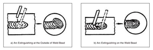
Fig 23 Arc Extinguishing Modes
