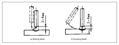
Fig 20 Arc Extinguishing Modes
