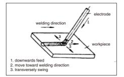
Fig 21 Three basic movement directions of electrode
