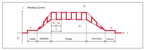
Fig 15 DC Pulse TIG Current Change Waveform
