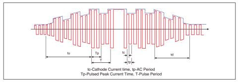
Fig 17 AC Pulse TIG Current Change Waveform
