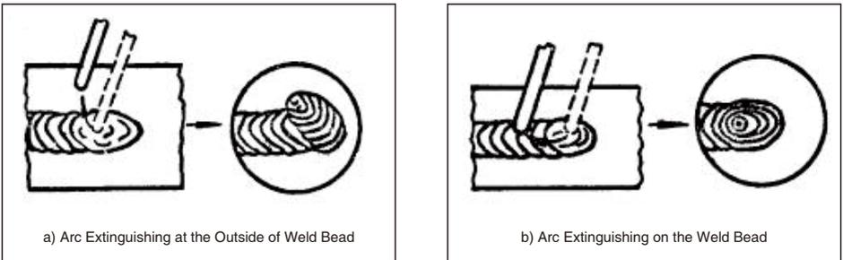
Fig 23 Arc Extinguishing Modes
