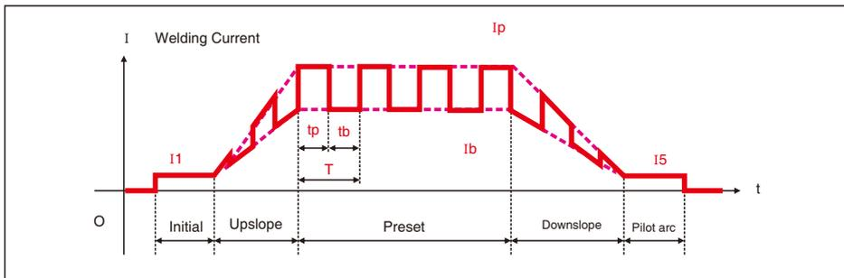
Fig 15 DC Pulse TIG Current Change Waveform
