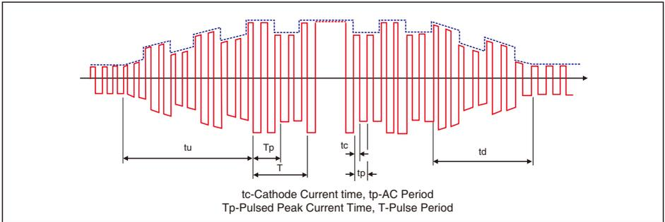
Fig 17 AC Pulse TIG Current Change Waveform
