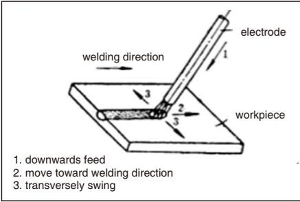
Fig 21 Three basic movement directions of electrode
