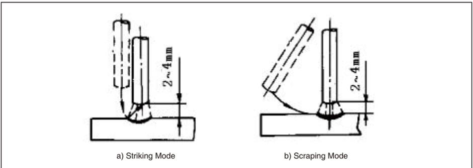
Fig 20 Arc Extinguishing Modes
