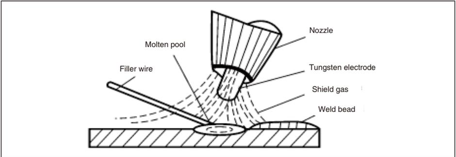
Fig 24 Sketch Map of Argon Arc Welding
