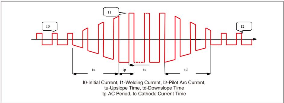
Fig 16 AC Square Wave TIG Current Change Waveform
