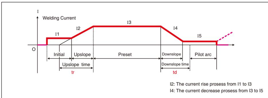
Fig 14 DC TIG Current Change Waveform
