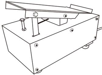
Fig 27 Pedal Remote Controller
