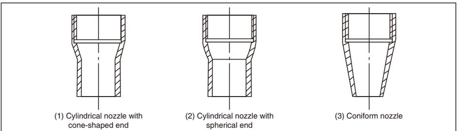
(1) Cylindrical nozzle with cone-shaped end
