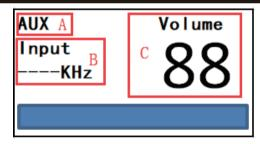
Input channel display area, USB/Optical/Coaxial/AUX/BT Input sampling rate area, no signal will show Volume display area, Volume range 0-99 At the bottom is the volume progress bar
