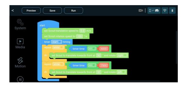
This graphical program generates Python codes and runs on Scout's ROS system. The Scout Scratch modules are divided into several categories, System, Media, Motion Control, Ai functions, Logic, Math, Loops, Lists, and Variables. Among them, Logic, Math, Loops, Lists, and Variables are standard modules by Blockly.
