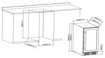
• For free standing installation, suggest to allow 2 inches of space between the unit's side, rear and the wall. In addition, sufficient clearance (160°) should be maintained to allow the glass door to open properly and completely.
