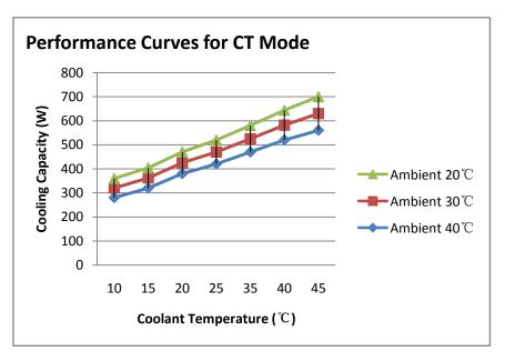
Note: Result was obtained with 150CFM air flow through condenser.
