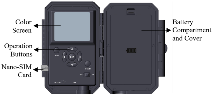
Figure 4: Inside View and Preinstalled SIM card
