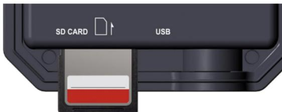
Figure 7: Inserting the SD Card
