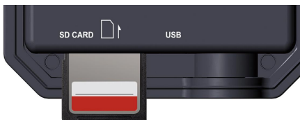
Figure 7: Inserting the SD Card
