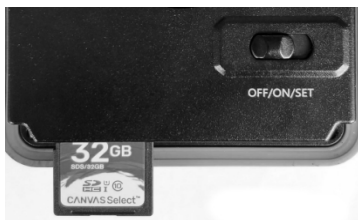
Figure 7: Inserting the SD Card
