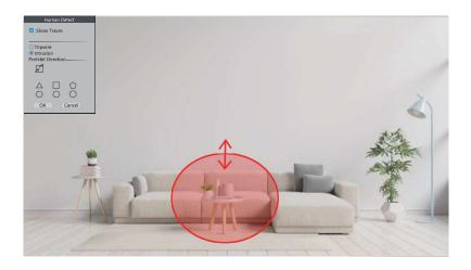
When we choose "Tripwire" in stead of "Intrusion", there will be a line on the screen and the camera will only detect or sound alarm when people cross this line.
