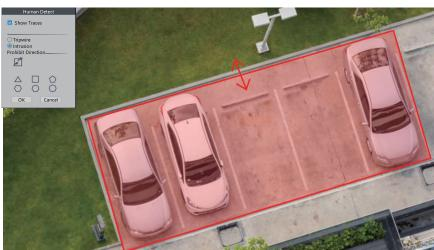
Click & hold the sides of the triangle then drag the sides to change the shape and the size of the safe zone.
