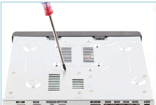
③ Screw HDD to the bottom
