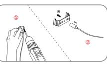
Secure suspended mounting kits to ceiling using 6-12 screws. Secure another side of suspended mounting kits to clips using 4-8 screws.
