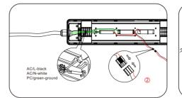
After the connection is completed, tighten the waterproof plug. Reconnect the wiring between the LED board and the driver.
