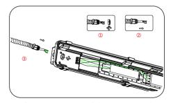
4. Separate the waterproof plug, and connect the input wire to the output wire of the power supply after passing through the plug and the outlet as shown in the figure.
