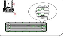
2. Release latches by pulling top of latch away from housing. Gently squeeze the buckle in and take out the PCB board (be careful not to touch the LEDs)..
