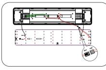
Disconnect the wire connecting the LED board and the driver to avoid unstable connection due to heavy suspension.
