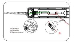
After the connection is completed, tighten the waterproof plug. Reconnect the wiring between the LED board and the driver.
