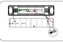
3. Disconnect the wire connecting the LED board and the driver to avoid unstable connection due to heavy suspension.
