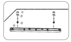
Secure suspended mounting kits to ceiling using 6-12 screws. Secure another side of suspended mounting kits to clips using 4-8 screws. Orient the luminaire so conduit fitting faces incoming supply power or conduit. Align the recesses and apply gentle upward pressure to secure luminaire onto both mounting clips.
