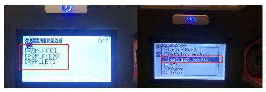
3/ To write the firmware of the R9MM receiver, you need to remove the R9MM receiver, and then write the firmware by connecting to the S.PORT port.
