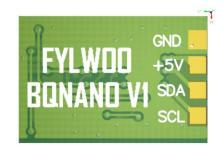
If your FC board has a barometer, you need to disconnect the Baro SDA / SCL pad. Baro/SDA
