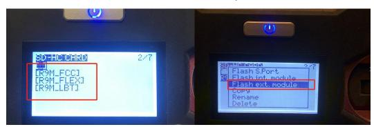
3/ To write the firmware of the R9MM receiver, you need to remove the R9MM receiver, and then write the firmware by connecting to the S.PORT port.
