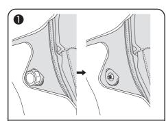
Remove the knob that is temporarily installed on the machine body.
