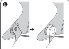
Attach the knob that was removed in Step 1.
