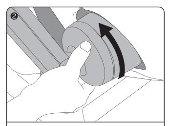
Insert the protrusions of the tablet stand connector to the three holes on the connector on the main machine (A, B, and D on the figure above), and then turn the connected part counterclockwise while depressing the Unlock button until the clicking sound is heard.
