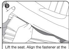
Lift the seat. Align the fastener at the upper end of the foot rest cover with that on the main body, and close the fastener.
