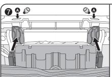
With the thread holes of the foot rest fulcrum shaft facing upward, lift the foot rest and set the foot rest fulcrum shaft to the foot rest fulcrum shaft receivers of the main machine. Mount the foot rest to the main machine by using the mounting screws at the portions **A**.
