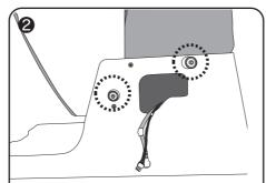
By using the supplied T-shaped wrench, remove the arm rest mounting screws (two pieces) that are temporarily attached on the machine body.
