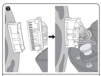
Connect the connector on the tablet stand (C in figure above) to the connector on the left side of the main machine. Align the claw direction with the counterpart and securely insert the connector.
