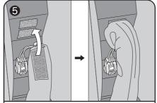
Tightly connect the air hose, and secure its upper part with a hook and loop fastener to fasten the hose.
