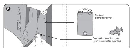
Put the foot rest cover on the foot rest while pushing the claws at two locations into the holes of the main machine, and then insert the push turn rivet to fasten the cover.
