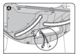
In the mounting in Step 3, pass the connector and air hose extending from the machine body through the take-out hole of the arm rests.
