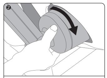
Turn the connected part clockwise between the tablet stand and the main machine while depressing the Unlock button to detach the tablet from the main machine.
