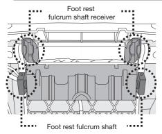
The right foot rest fulcrum shaft receiver and the left one differ from each other. Check the difference before starting work.
