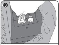
Positively insert the cloth-covered connector on the foot rest side to the main machine side until a clicking sound is heard. Insert the connector with its claw side facing outward.
