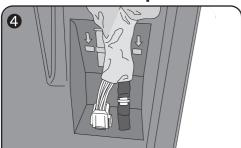
When attaching the air hose, confirm that the relay hose covered with cloth is not forcefully twisted.
