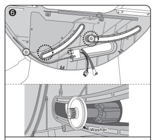
After attaching the knob, securely tighten the arm rest mounting screws at the two locations that were removed from in Step 2, by using the T-shaped wrench to fasten the arm rests.
