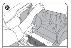
By using the supplied T-shaped wrench, securely fasten the foot rest with the foot rest mounting screws. (Although the figure illustrates the right side of the seat, also work in the same way for the left side.)
