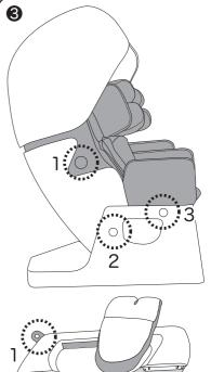
Insert the arm rest into the machine body (at three locations). \*Pay attention not to pinch the connector and air hose.
