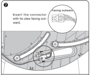
Connect the connector and air hose extending from the machine body that were taken out in Step 4 to the connectors that are fixed to the arm rest. Fully insert them until a clicking sound is heard.
