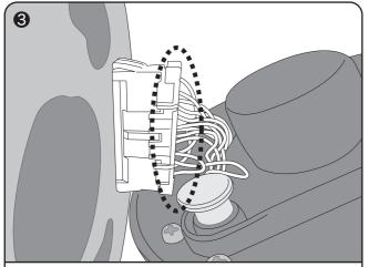
To disconnect the connector, hold down the connector edge with your finger to disengage the claws, and then pull the connector.
