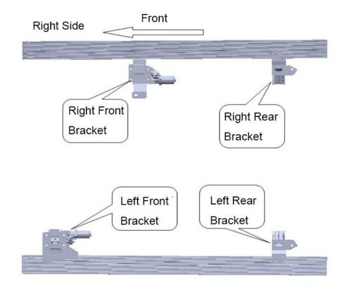
2.Remove the guard plate of car chassis and find out factory holes.And then remove the rubber plugs and rivets of these holes.Please don't tighten all screws firstly.
